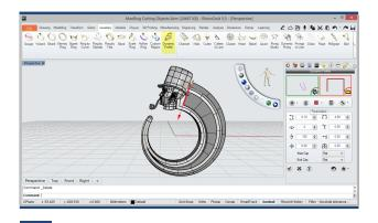
Dynamic Profile Now, we'll define a dynamic profile applying on the Extracted curve in the previous step to use it as the cutting object, we'll respect a margin of 1mm to the initial dynamic profile.
