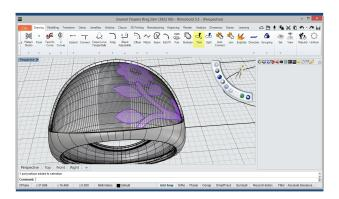
In this step, we'll select the Trim tool and apply it between the projected curves and the extracted surface.
