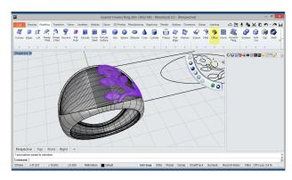
Then, we'll apply the Offset tool to the new surface obtained in the previous step, with 0.5 mm distance.
