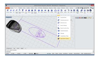
Apply Border in Surface Then, we'll select the Apply Border in Surface tool, in the Duplicate Edge submenu, and apply it between the curves of the plane and the ring surface, as shown in the picture.
