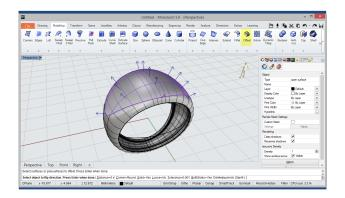
Offset Then, we'll apply the Offset tool in the new surface obtained with the previous step, applying a distance of 0.4 mm. We'll make a copy of the offset surface and keep hidden for future operations.
