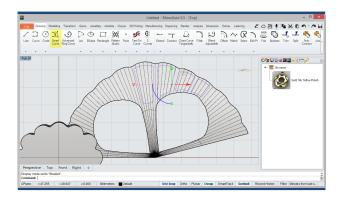
In this step, we'll trace four closed similar curves to those shown in image, using the Smart Curve tool.
