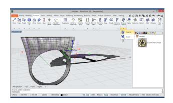
Flow by Surface Then, we'll project the flat surface curves on the ring surface, with the Flow by Surface tool.
