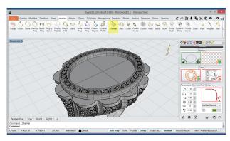
18 Then, we'll select the Channel tool, at the Jewellery tab and define a channel with gems of 1.30 mm, positioning it on top of the ring. We use the initial Ellipse to define the channel.
