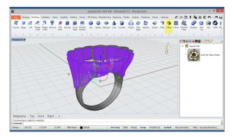
In this step, we'll select the Offset tool, in the Modelling tab and apply it an offset of 0.3 mm on both sides of the surfaces.
