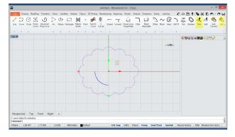
Now, we'll go to the Drawing tab and apply the Trim tool between the curves of the array, obtaining the same result as in the image. After we'll unite the curves with Join tool.
