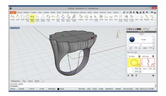
Signet Ring Then, we'll define a ring with the Signet Ring tool, in Jewellery tab. Apply the curve saved in the User Folder, clicking on the option of top profile in the tool
