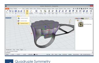
Now, we'll apply a Symmetry to the projected curves with the Quadruple Symmetry tool.
