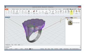
10 Then, we'll select the Trim tool and will apply it between the extracted surface and projected curves, getting the inside surfaces of the curves.
