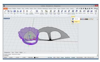
Extract Surface / Smash Now, we'll duplicate the lateral surface of the ring with the Extract Surface tool, within the submenu Cap, at the Modelling tab. Then we'll go to the Transform tab and apply Smash tool to the extracted surface.
