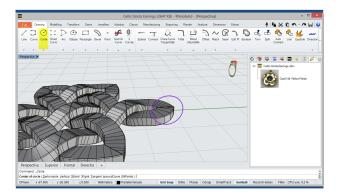
Circle Next, we define a circle to the top knot with the Circle tool, on the Drawing tab, as shown in the image above.
