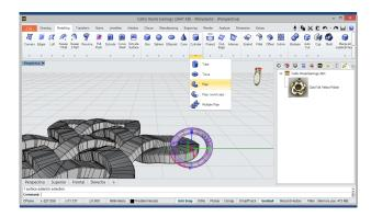
Pipe In this step we will apply the Pipe tool to the circle created earlier. This tool is located within the cylinder submenu in the Modelling tab.
