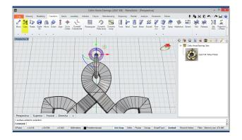
Сору Now we copy the pipe from the previos step with the Copy tool, in the Transform tab and will position as shown in the image.
