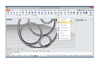
Extract Isocurves Now, we will select the Extract Isocurve tool in Duplicate Edge submenu in the Model tab, and apply it to the dynamic profiles previously created, extracting curves.
