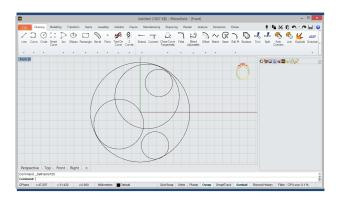
First, we will create four similar circumferences to the image, with the Circle tool. We will reference the largest circle that measured 30 mm in diameter and we will position it as shown the image.
