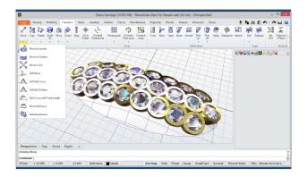
In this step we will use the original surface created to support the Pave. Under the Transform tab we will choose the Move tool to place it down 0.8mm under the original position.
