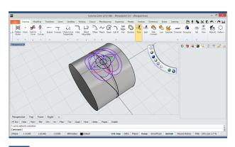
Now, we'll apply the Trim tool between the offset curves and the extracted surface.
