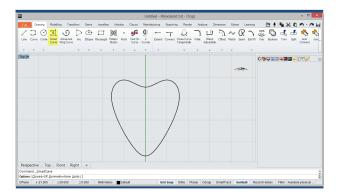
**Smart Curve** Then, we'll select the Smart Curve tool, in the Drawing tab and will trace a similar curve to that shown in the image.
