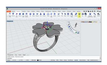
Now, we'll select the Auto Cut tool, in the Modelling tab and apply it between the gem curve and the extruded surface.
