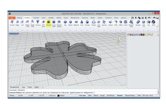
Extrude In this step, we'll apply the Extrude tool to the curve, in the Modelling tab. We'll define a Extrusion of 2mm.
