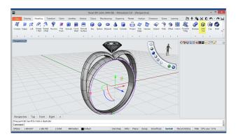
Then, we'll select the first Gauge curve and Shank and will apply the Auto Cut tool, in the Modelling tab.
