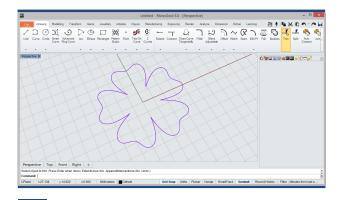
Trim/Join Then, we'll apply the Trim tool, in the Drawing tab to remove intersecting curves of the Array. Then apply the Join tool to the curves.
