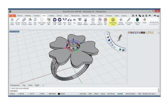
Extract Gem Curve Then, we'll extract the diameter curve of the gem with the Extract Gem Curve tool, in the Gems tab.
