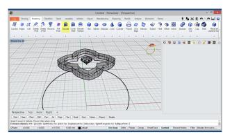
Extrude Then, we'll select the Extrude tool in the Modelling tab and apply an extrusion of 1mm, keep the "BothSides" option Off and "Solid" activated in the command line.
