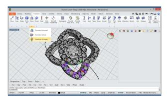
Quadruple Symmetry/Boolean Union Now, we'll apply a Quadruple Symmetry to the prongs defined in the previous step and apply a
