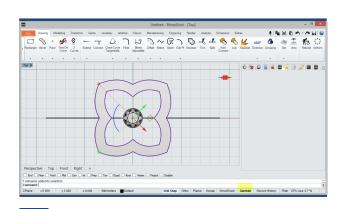
Gumball Now, we'll rotate 90° the extruded solid and curves, with the Gumball command.
