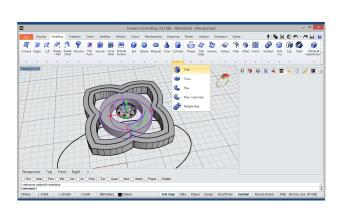
Now, we'll go to the Modelling tab and select the Tube tool, define a solid 1mm in width and height, as shown in the picture.
