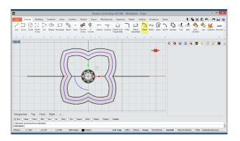
Next, we define a middle curve of 0.5mm between the created curves, with the Offset tool.
