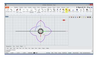
Join Now, in the Drawing tab, we'll select the Join tool and apply it between the two curves created in the previous step, obtaining a single curve.
