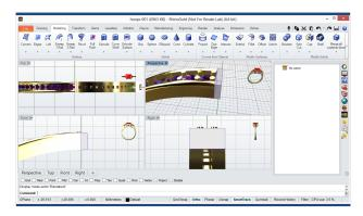
Box Now, under the Modeling tab we will use the Box command to create an object as seen in the above image which will support the ear wire.
