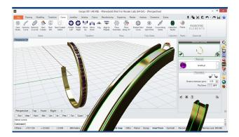
Gems by 2 Curves Now, in the Gems tab, run the Gems by 2 Curves tool and define the parameters to place the gems around the hoop. Select the inner edges and click preview.
