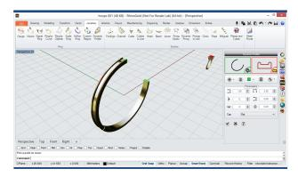
Dynamic Profile Now, under the Jewelry tab with the Dynamic Profile tool select the arc and define all the parameters to create the hoops according to our needs. We recommend 1.5mmx2.5mm dimentions of the profile
