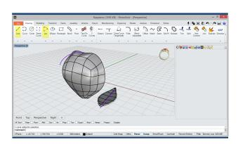
Arc/Line In this step, we'll define two curves, an arc positioned at the top of the first solid and a straight located below the last solid, as shown in the image.
