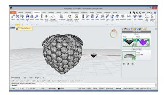
Copy by Gems Now, select the Copy by Gems tool, in the Transform tab and apply between gems created in the previous step and Pavé gems, as shown in the image above.
