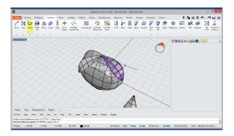
Rotate Then, we'll select the Rotate tool and we'll apply it the above solid, with the copy option activated on the command line.
