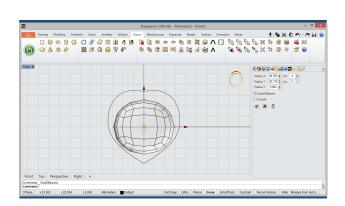
Clayoo: Sphere In this step, we will go to Clayoo tab and we'll activate it then define a solid with the sphere tool.
