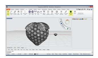
Gem Studio/Cabochon Studio In this step, we'll define a Gem of 5 mm in diameter with a Cabochon located above the same diameter and 2mm high. These gems we'll define it with the-Gem Studio tool and Cabochon tool, within the Gem tab.
