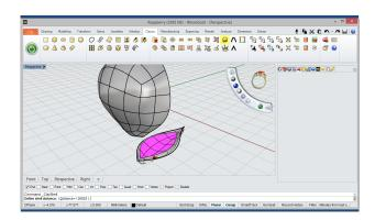
Clayoo: Shell After we'll apply the Shell tool to the surface created in the previous step, define a thickness of 1 mm.
