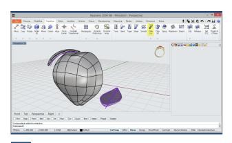
Flow Curve 15 Then, we'll select the two curves created in the previous step and the last solid created and apply the Flowing Curve tool, obtaining the same result as shown in the image, the second solid above the first.
