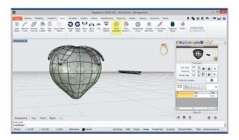
Pave Automatic Then, select the Pavé Automatic tool in the Gems tab and apply it in the first solid created with gems of 5 mm in diameter.
