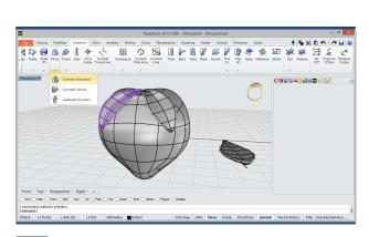
Simmetry Horizontal Now, we'll apply a Symmetry Horizontal at the solid positioned at the top. It is important that all solid are touching each them.
