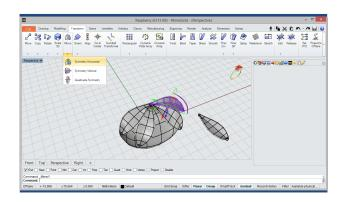
Symmetry Horizontal Now, we'll apply a Symmetry to the solid copied, obtaining a result as shown in the image.
