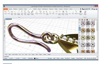
Lastly under the Jewelry tab with the Findings tool define the earrings wire. We can activate the Gumball transformer to adjust the positions and measurements, as shown in the image above.
