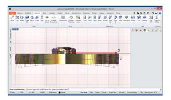
Bend In the front view with the Bend tool, under the Transform tab we can adjust the leaf shape as seen in the above image. It's important to activate the symmetry option in the command line.
