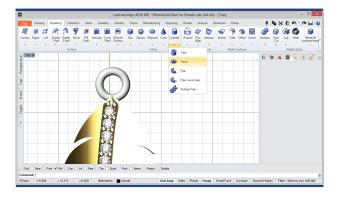
Torus / Boolean Union 13 Now, in the top view, with the Torus tool under the Modeling tab define a shape to support the earrings wire. Then, with the Boolean Union tool under the Modeling tab unite all the metal parts into a single object
