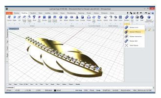
Boolean difference With the Boolean Difference tool under the Modeling Tab remove all of the Cutters on the leaf earring.
