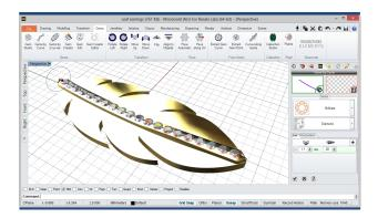
Gems by Curve We can apply gems along the curve, for this, under the Gems tab use the Gems by Curve tool, in this case with 20 x 1.10mm gems.
