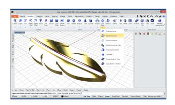
Extract Isocurves Back to the Modeling tab with the Extract Isocurves tool we can get the central curve from the surface created in step 5. It's important to activate the Mid option under the Osnap.
