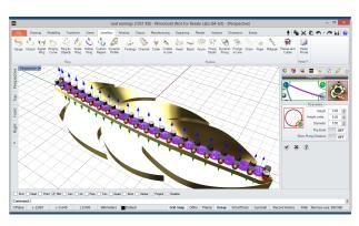
Prongs in Line 10 Now we should create the prongs to support the gems, for this, use the Prongs In Line Tool under the Jewellery tab and define the intended parameters. We can then use the Prong Editor tool to adjust some parameters if need be.
