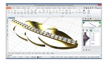
**Cutter Studio** Under the Jewelry Tab with the Cutter Studio tool define all of the parameters of the cutters that will be applied onto the gems as the above image.
