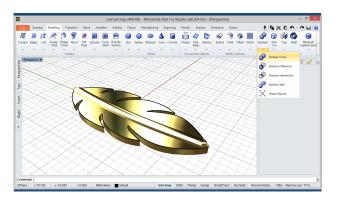
**Boolean Union** We can then use the Boolean Union tool under the Modeling Tab to unite both parts into a single object as shown in the image above.
