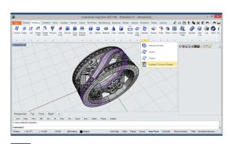
Average 2 Curves on Surface Now, we'll apply the Average 2 Curves on Surface tool to extract the central curve of the bridge, located in the Intersect submenu, in the Modelling tab.
