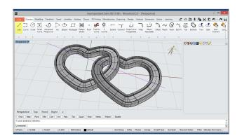
Then, we'll trace a curve through the two Dynamic Profiles with the Line tool, in the Drawing tab.
