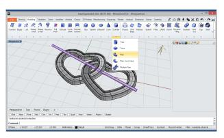
In this step, from the Modelling tab, we'll define a solid of 1mm with Pipe tool, selecting the curve of the previous step.
