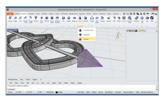
In this step, we'll define a pyramid-shaped solid and will position it at the end of the pipe, we'll use the Pyramid tool, within Cone submenu, in the Modelling tab.
