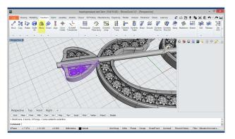
Now, we'll apply a Symmetry to the extruded solid at the extreme from the Transform tab.
