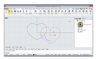
Then, we'll make a copy of the curve with the Copy tool, in the Transform tab. We'll position the new curve in the same manner as in the image.
